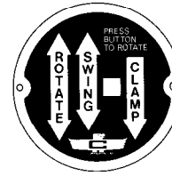
A Visible on trucks with a single handle controlling auxiliary valves
