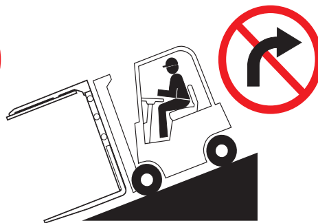
No turning on ramp
