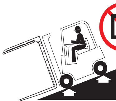
No parking on ramp
